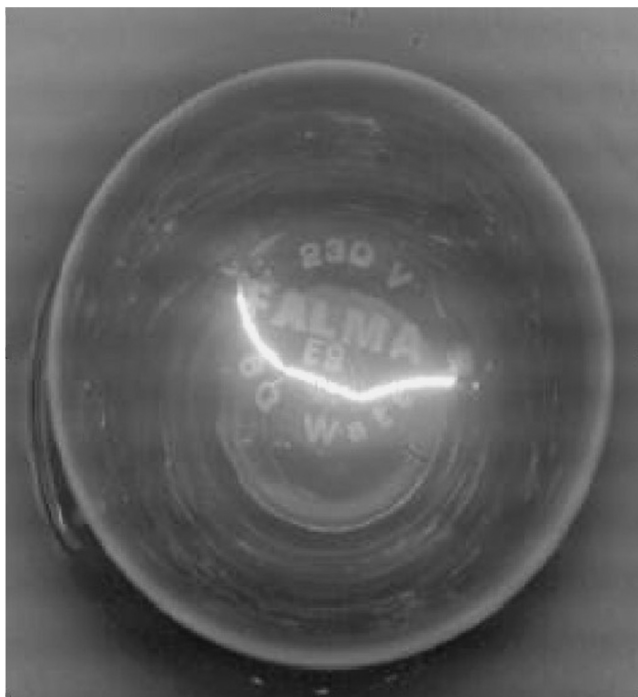
Figure 1.3 Image of a lightbulb using a logarithmic sensor with off-chip fixed-pattern noise correction (courtesy of Dierickx [83]).
