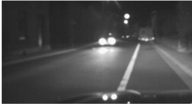
Figure 1.2 Example of an HDR automotive front-vision application. The image was acquired in 2004 with an early-model panoramic VGA global shutter automotive image sensor.
