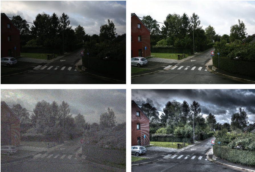
Figure 1.17 Post-processing attempts of the last, non-saturated picture of Fig. 1.13 compared to an HDR version of the same scene taken with the same camera and the same saturation level. Top left: original image. Top right: gamma. Bottom left: strong sharpening. Bottom right: HDR merged and tone-mapped image.
