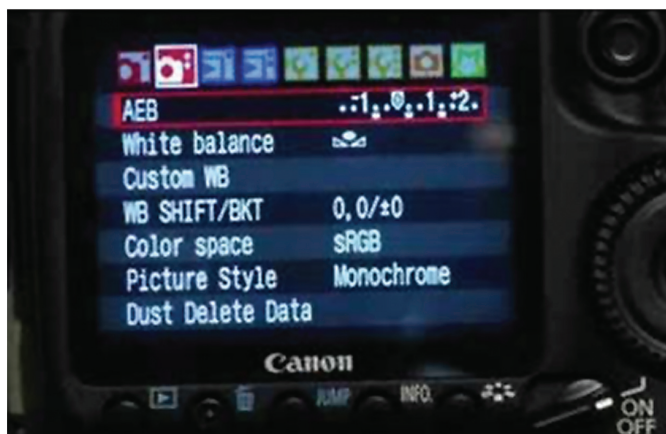
Figure 1.11 Exposure menu of the Canon EOS 40D, showing the exposure bracketing settings (AEB).
