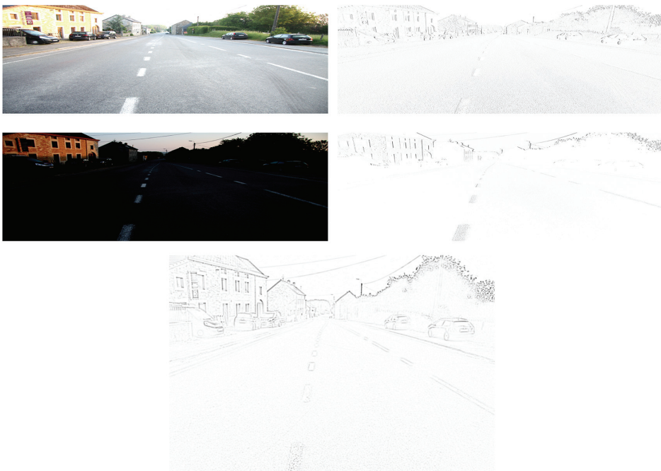
Figure 1.18 Road-marking-detection algorithm in an HDR scene without HDR imaging. Top left: even lines, long exposure. Top right: result of a horizontal edge detector on long-exposure lines. Middle left: odd lines, short exposure. Middle right: result of a horizontal edge detector or short-exposure lines. Bottom: combined and filtered binary edge image.
