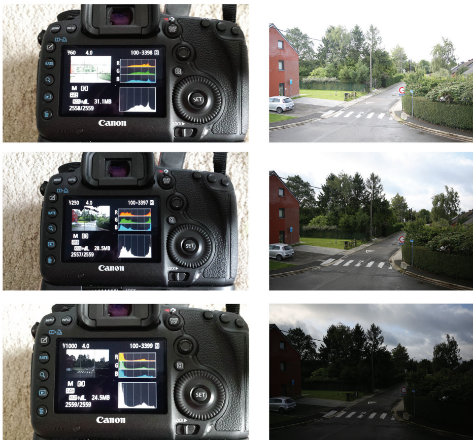
Figure 1.13 Adjustment of the exposure of a Canon EOS 40D based on histograms until the image is no longer saturated. The exposure time can be seen in the top-left corner of the screen.
