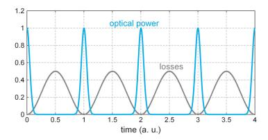
After thousands of round-trips, a steady state is reached where this shortening effect is balanced by pulse-broadening effects (for example, the limited gain bandwidth or chromatic dispersion). The pulse duration of actively mode-locked solid-state lasers is typically a few tens of picoseconds. This means that the pulse bandwidth is far smaller than the gain bandwidth of the laser medium.
