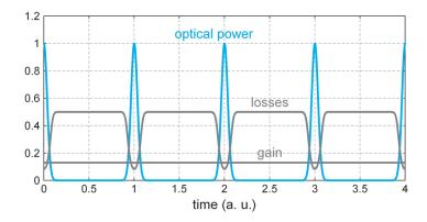
As shown in the figure above, the pulse experiences higher losses in its wings, compared with the peak. In that way, the absorber tends to temporally shorten the pulse. In addition, the absorber serves to suppress any temporally broad background or weak satellite pulses, and thus stabilizes the circulating pulse.
