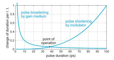
The major pulse broadening effect is often spectral gain narrowing, caused by the finite gain bandwidth of the laser medium. In that situation, it is relatively simple to calculate the pulse duration in the steady state, as was first done by Kuizenga and Siegman (Ref. Kuizenga and Siegman 1970). The result is
