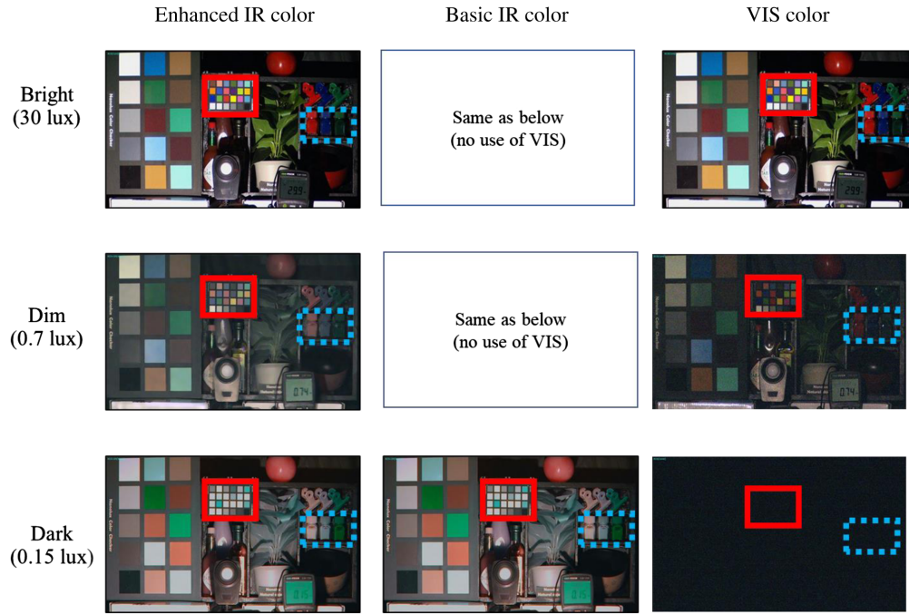
Fig. 8 Enhanced IR color, basic IR color, and VIS color by illumination level.
