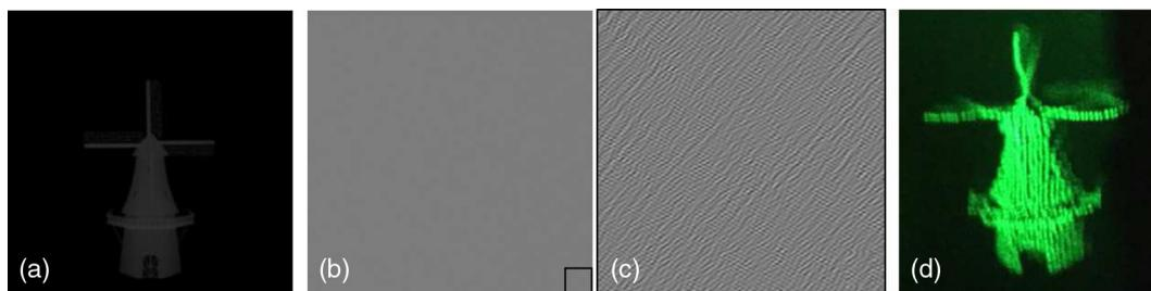
**Fig. 4** 3D object video used in our experiments. (a) 46th frame, (b) its CGH image ( $1536 \times 1536$ ), (c) enlargement of a region (black square) in the CGH image, and (d) the optical reconstruction image. The main purpose of this study is the rapid generation of the CGH image for each frame.
