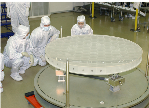
Fig. 2 Kepler's 1.4-m-diameter, f/1 primary mirror is made of Corning ULE®. It was fabricated and polished by L-3 Integrated Optical Systems (formerly Brashear). The water-jet cut core achieved 88% light-weighting, for an areal density of 48 \text{ kgm}^{-2} , and a mass of 86.3 kg.
