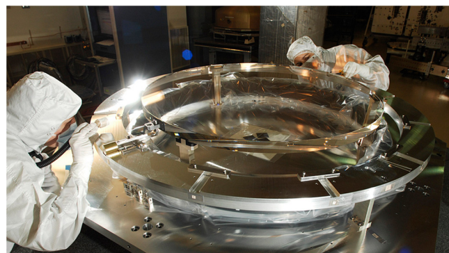
Fig. 4 The Corning fused silica, plano-convex Schmidt corrector was fabricated by L-3 Integrated Optical Systems (formerly Brashear and Tinsley). Here it is being prepared for bonding of its support flexures at Ball Aerospace.
