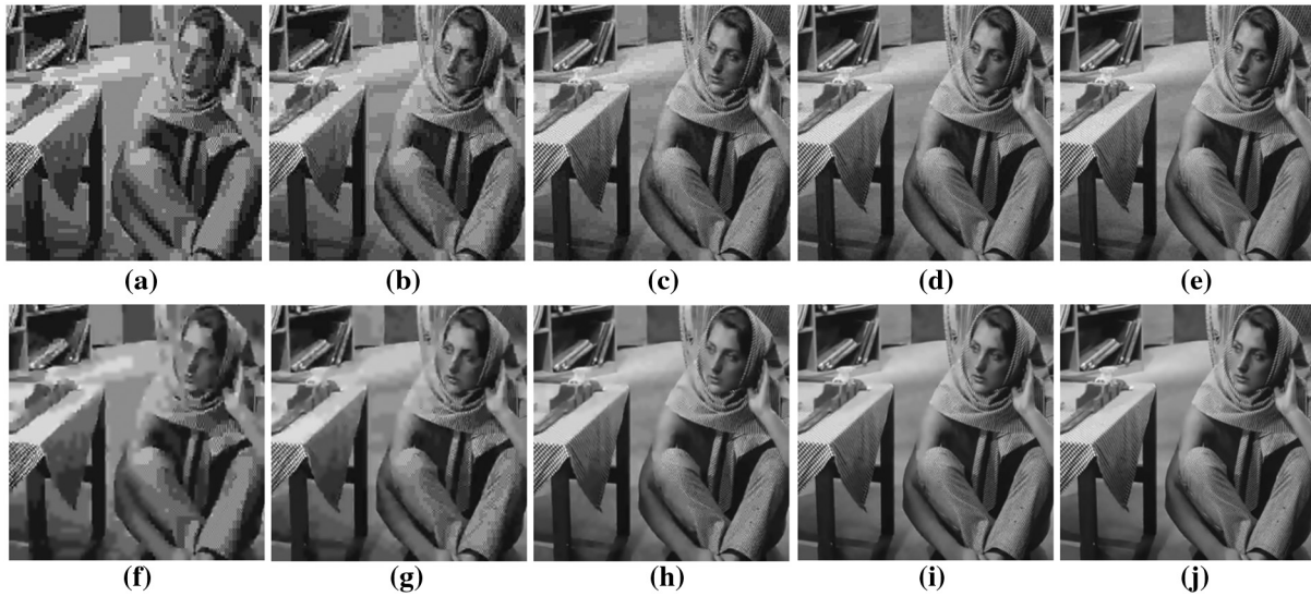
Fig. 12 JPEG compressed images and their deblocked results of the Barbara image according to different quality values: (a) quality = 1, (b) quality = 5, (c) quality = 10, (d) quality = 15, (e) quality = 20, (f) the deblocked result of (a), (g) the deblocked result of (b), (h) the deblocked result of (c), (i) the deblocked result of (d), and (j) the deblocked result of (e).
