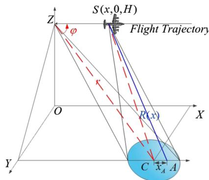
Fig. 1 Acquisition geometry of airborne squint spotlight synthetic aperture radar (SAR) mode.
