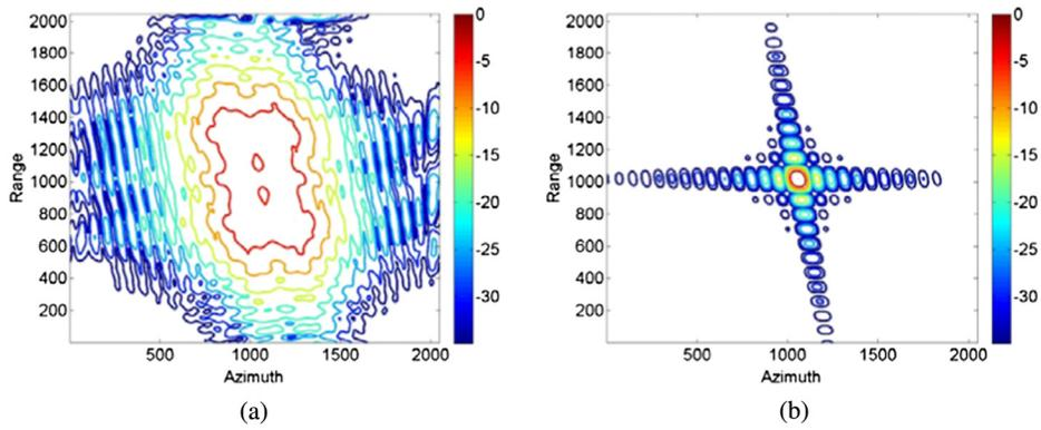
**Fig. 8** Comparing imaging results of conventional WDA and improved algorithm. (a) Conventional WDA. (b) Proposed imaging algorithm.
