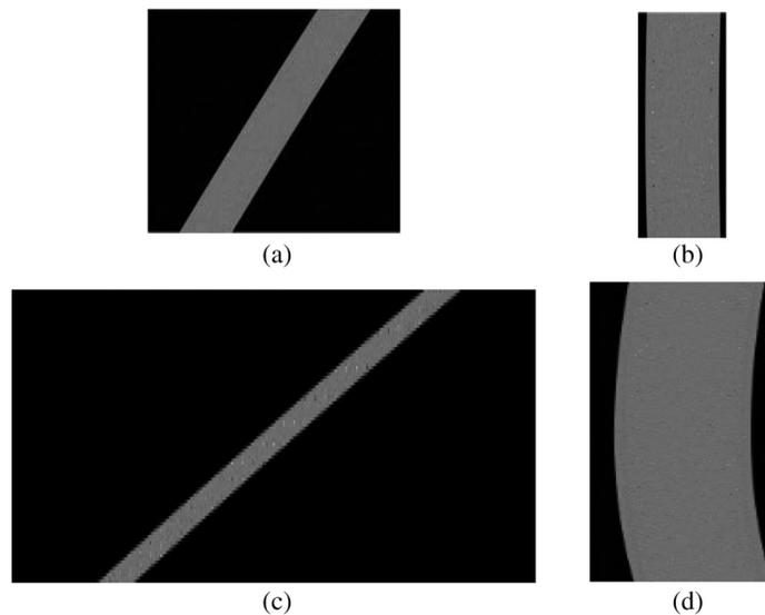
Fig. 7 Comparing the echo data of ASRW-SAR and conventional SAR systems at different squint angles. (a) conventional SAR,  $\varphi = 40 \times \text{deg}$ ,  $N_r = 32768$ , (b) ASRW SAR,  $\varphi = 40 \times \text{deg}$ ,  $N_r = 8192$ , (c) conventional SAR,  $\varphi = 70 \times \text{deg}$ ,  $N_r = 262144$ , and (d) ASRW SAR,  $\varphi = 70 \times \text{deg}$ ,  $N_r = 16384$ .
