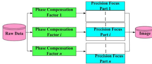
Fig. 5 Flowchart of block processing.
