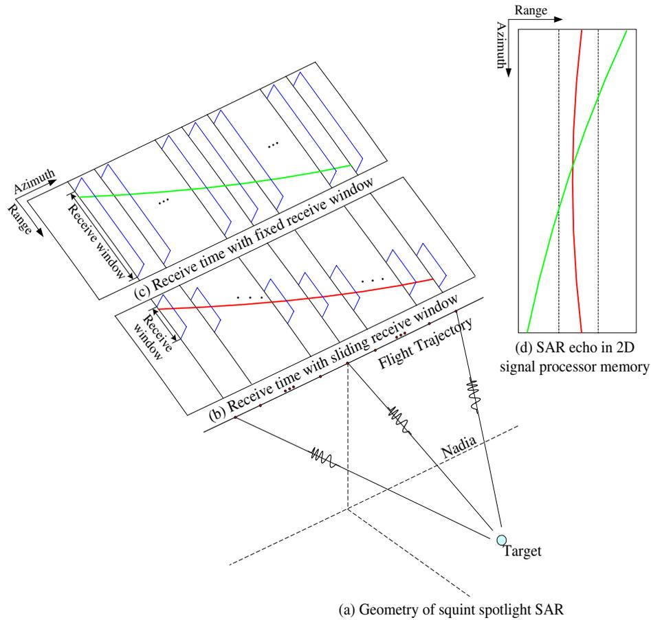
**Fig. 3** Operation mechanism for airborne squint spotlight SAR using adaptive sliding receive window (ASRW).
