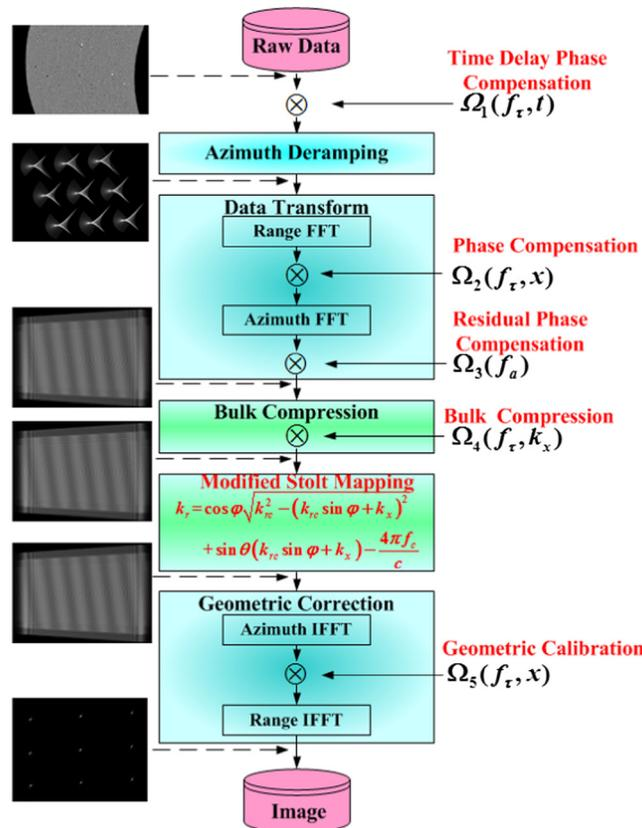
Fig. 4 Flowchart of the proposed wave number domain algorithm (WDA).
