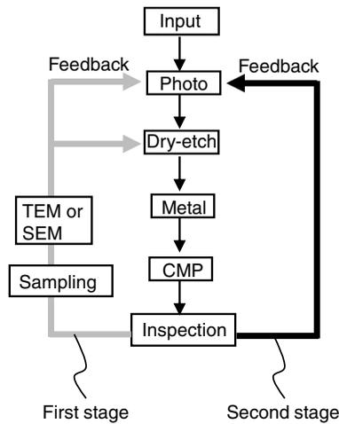
Fig. 1 Prospective process flow applying in-line resistance inspection.
