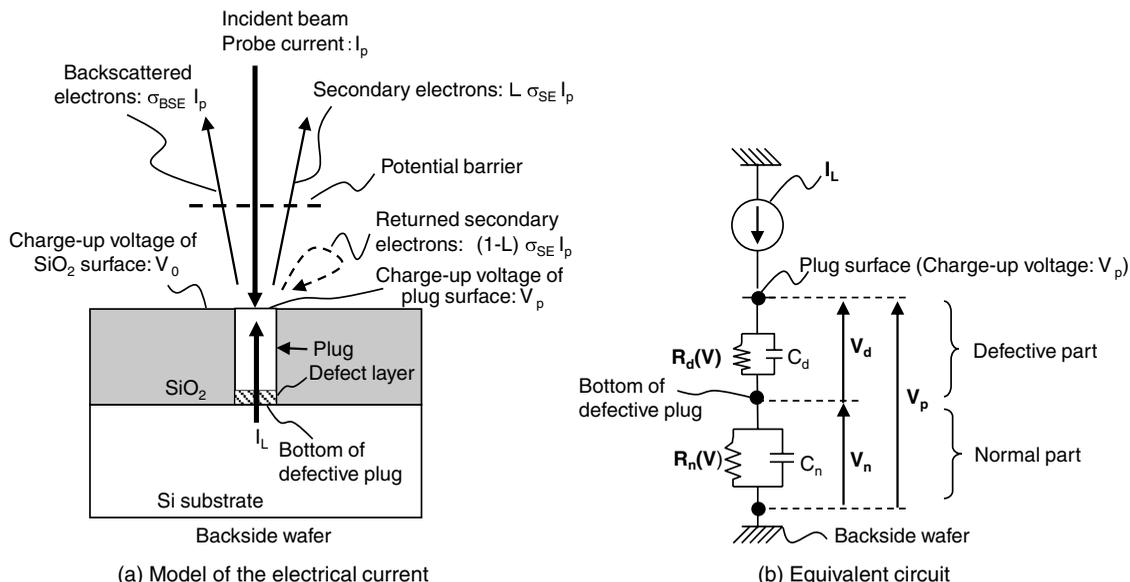
Fig. 2 Schematic illustration of the equivalent-circuit model.
