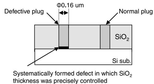
Fig. 4 Schematic cross section of a standard calibration wafer.
