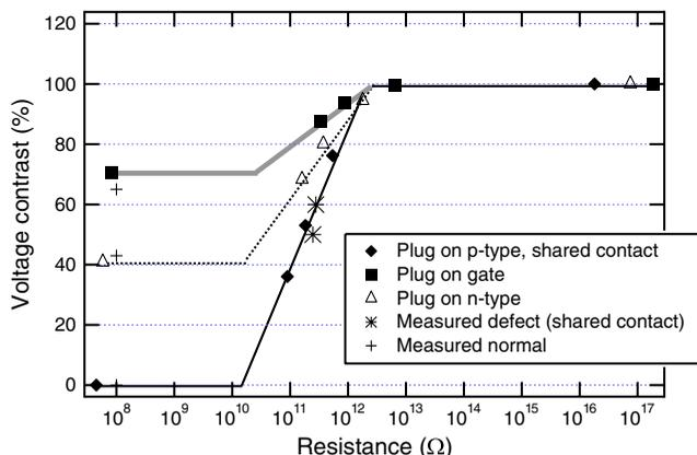
Fig. 10 Calibration curve for SRAM pattern.
