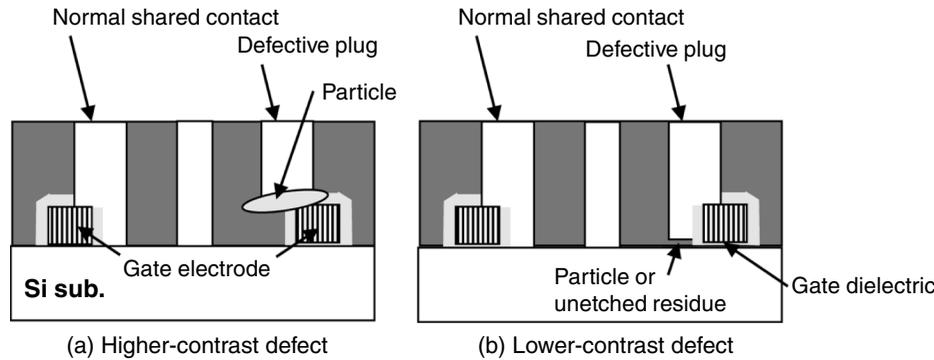
Fig. 13 Schematic cross-sections of a detected defect with higher contrast and a defect with lower contrast.
