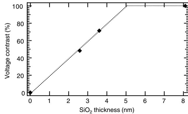
Fig. 9 Calibration curve for SiO<sub>2</sub> thickness at bottom of defect.
