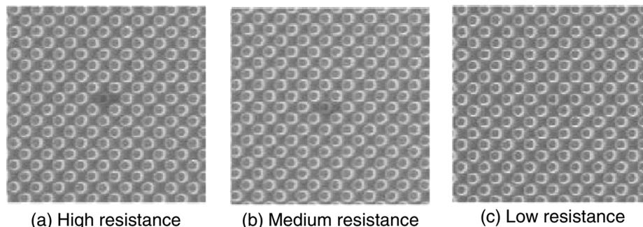
Fig. 7 SEM images of an intentional defect on standard calibration wafers.
