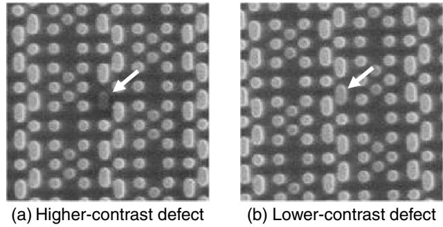
Fig. 11 Examples of SEM images of a defect with higher contrast and a defect with lower contrast on an SRAM wafer.
