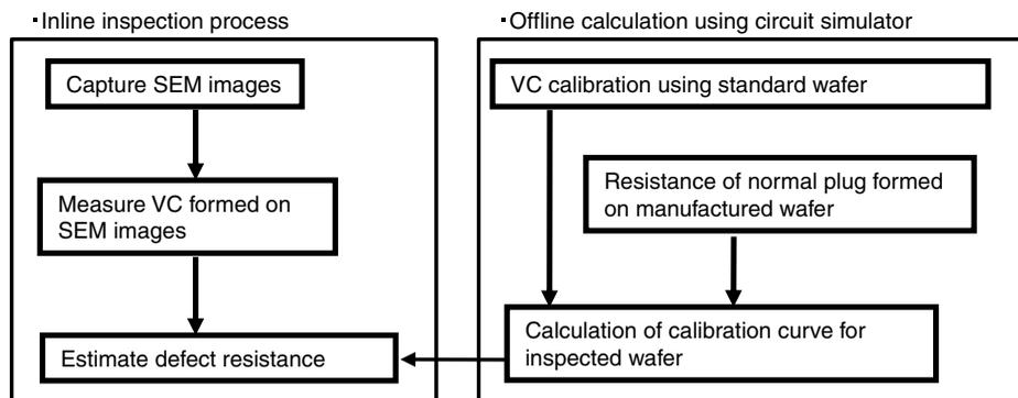
Fig. 3 Inspection process flow for estimating defect resistances formed on manufactured patterns in various devices.
