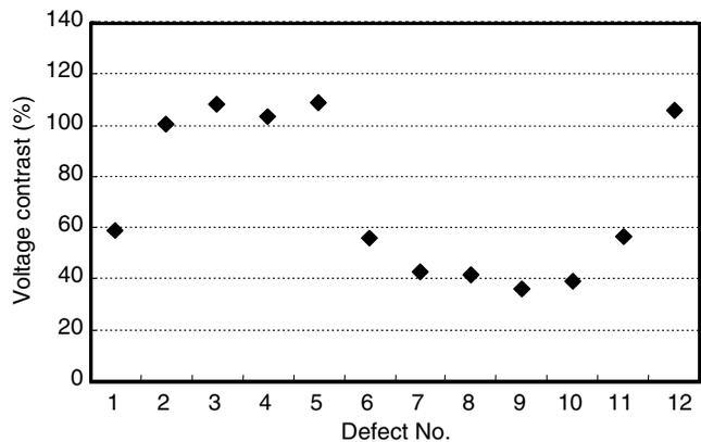
Fig. 12 Variation in voltage contrast measured from defect images formed on a plug for shared contacts. Voltage contrast is separated into two levels.
