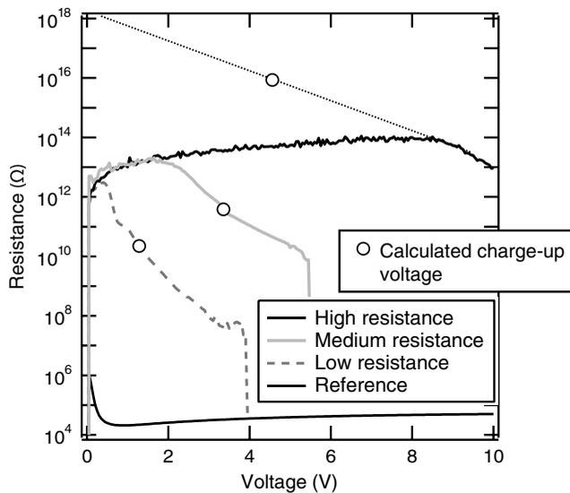
Fig. 6 Resistance of defects measured with a nano-prober as a function of differential voltage between W plug and Si substrate.
