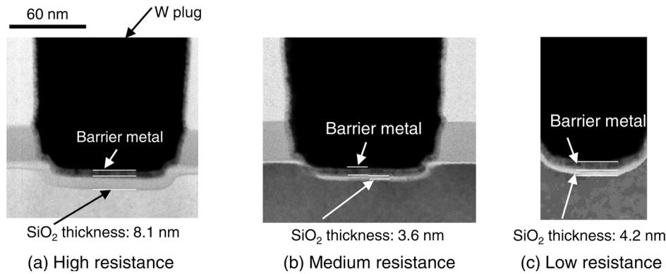
Fig. 5 Cross-sectional TEM images at the bottoms of the defective plugs with three varieties of resistances.
