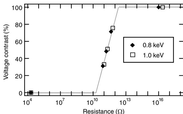
Fig. 8 Calibration curve obtained from the calculation considering measured I-V characteristics of defects formed on standard calibration wafers.
