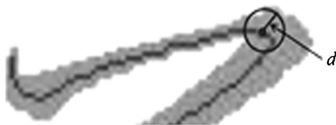
Fig. 9 Stroke thickness. Red pixels are the skeleton and the gray pixels are the foreground of a stroke. d is the radius of the maximal foreground disk, centered on a skeleton pixel marked with a darker dot.
