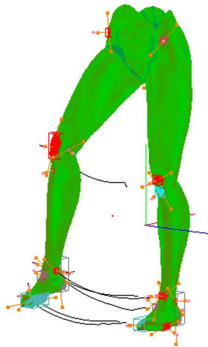
Fig. 16 Sample trajectories of groups related with a knee, malleoli, toes, and a heel calculated for computer-simulated data.
