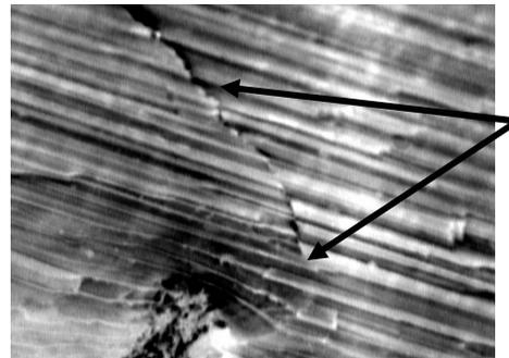
Fig. 21. Images of a disturbed part of a bariumtitanate single crystal (magnification 150x, image size about 800 x 800  $\mu\text{m}$ ). Left: conventional SEM image with secondary electrons. Right: SEAM with  $f = 119$  kHz.
