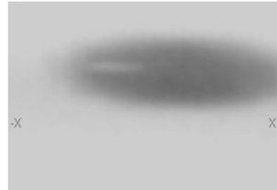
Fig. 11. Computer tomographic slice of a sample with a produced test flaw, which is clearly visible.
