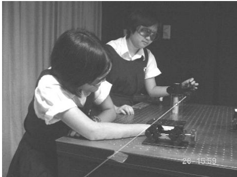
Fig.1 Students from RGSS using the spatial filter to align the beam.
