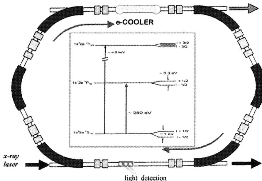
Figure 6: X-ray laser spectroscopy on highly charged heavy ions in the ESR. Due to the Doppler shift the photon energy can be matched precisely to the hyperfine transitions for example in lithium like uranium.
