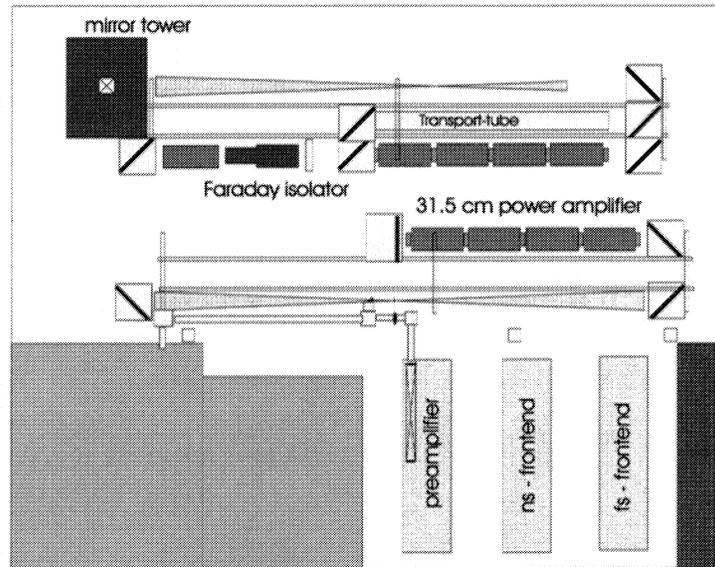
Figure 1: Layout of the PHELIX laser.
