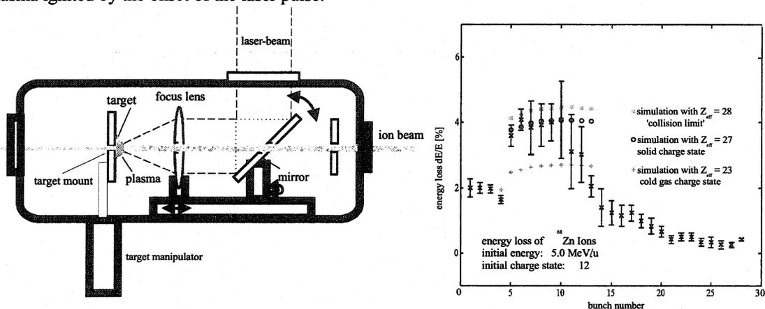
Figure 5: Heavy ion beam – plasma interaction experiments. Left: experimental setup. Right: energy loss measurement. After the constant energy loss in the cold matter (first 4 bunches), the enhanced energy loss is clearly visible. After 7 bunches (63ns) the energy loss is reduced due to hydrodynamic expansion of the target matter.
