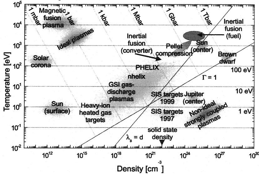
Figure 4: Astrophysical and laboratory plasma covering many orders of magnitude in density and temperature. The present and future experimental capabilities of GSI are shown.
