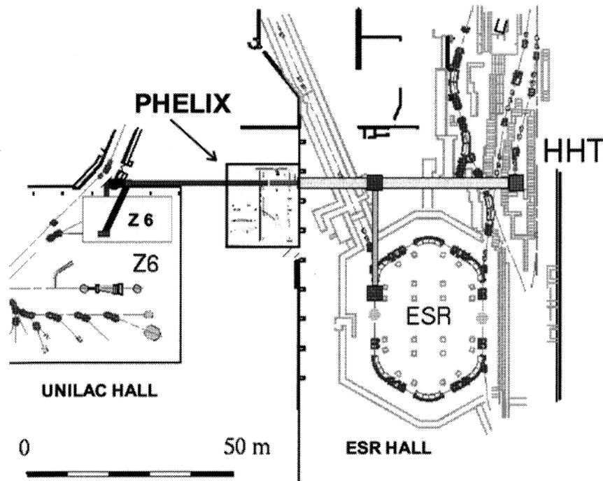
Figure 2: The PHELIX laser is integrated into the GSI accelerator structures to minimize the distance from the experiments and to keep the number of turning mirrors as small as possible.
