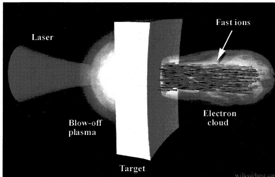
Figure 7: Sketch of the proton acceleration (by Wilks). The main laser beam is interacting with the blow off plasma produced by the pre-pulse. A large number of hot (several MeV) electrons are produced that penetrate the target and form an electrostatic acceleration sheath at the rear surface, where a steep density gradient results in accelerating fields of MV/ $\mu\text{m}$ .
