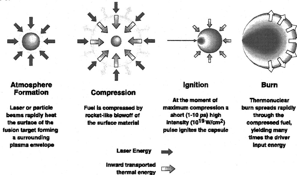
Figure 8: Diagram of Fast Ignition concept in inertial confinement fusion.
