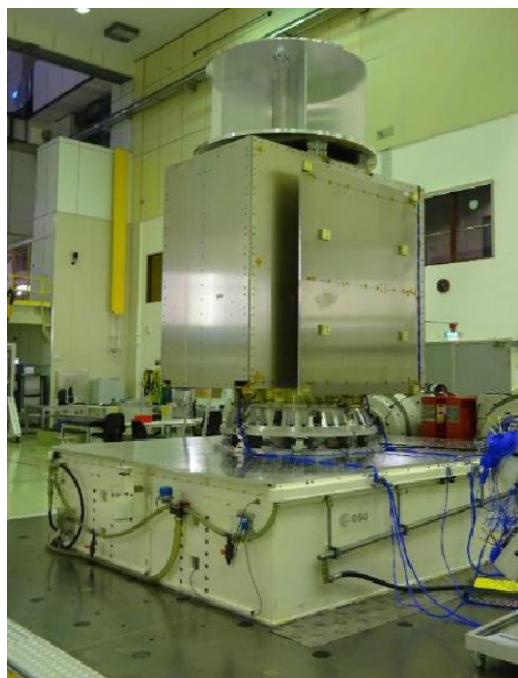
Figure 2: The Satellite Structural Model on the shaker at ESTEC/ESA
