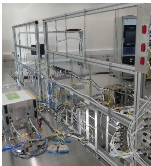
Figure 3: The Satellite Engineering Model with the first electrical units of the platform integrated
