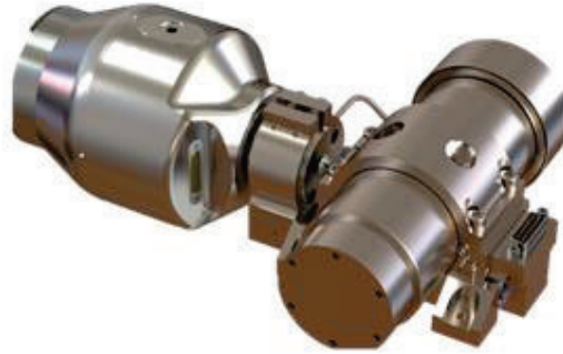
Figure 11. Active Detector Package composed of a Dewar and a LPT cooler for NGP and COBRA detectors.
