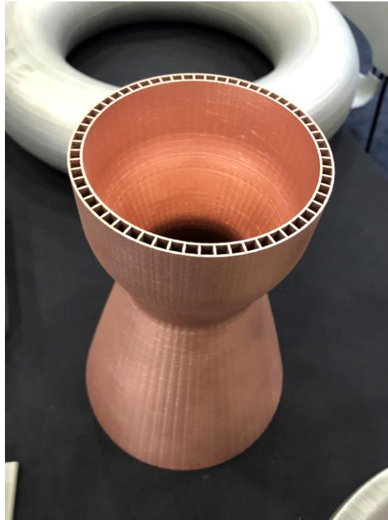
Figure 6. GR Cop 42 copper alloy rocket nozzle demonstrator processed by LMD using a green wavelength.
