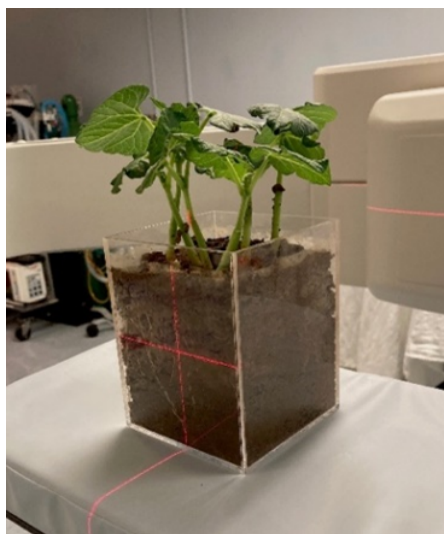
Figure 1. A sample of a root-soil system imaged to study soil aggregates.
