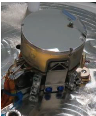
Figure 2-1: View on the difficulties of access to measure the mechanical reference frame after the final integration (M2 mirror FCI)
