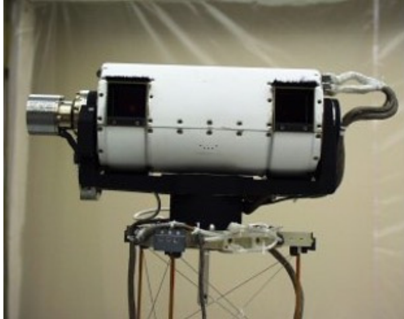
Figure 6. The IMP camera head at the top of its extendable mast. The two “eyes” allow for stereo views important for tracking the rover’s progress. The white cylinder is 8 inches long and the pointing is driven by two motors in an alt-az mount configuration.
