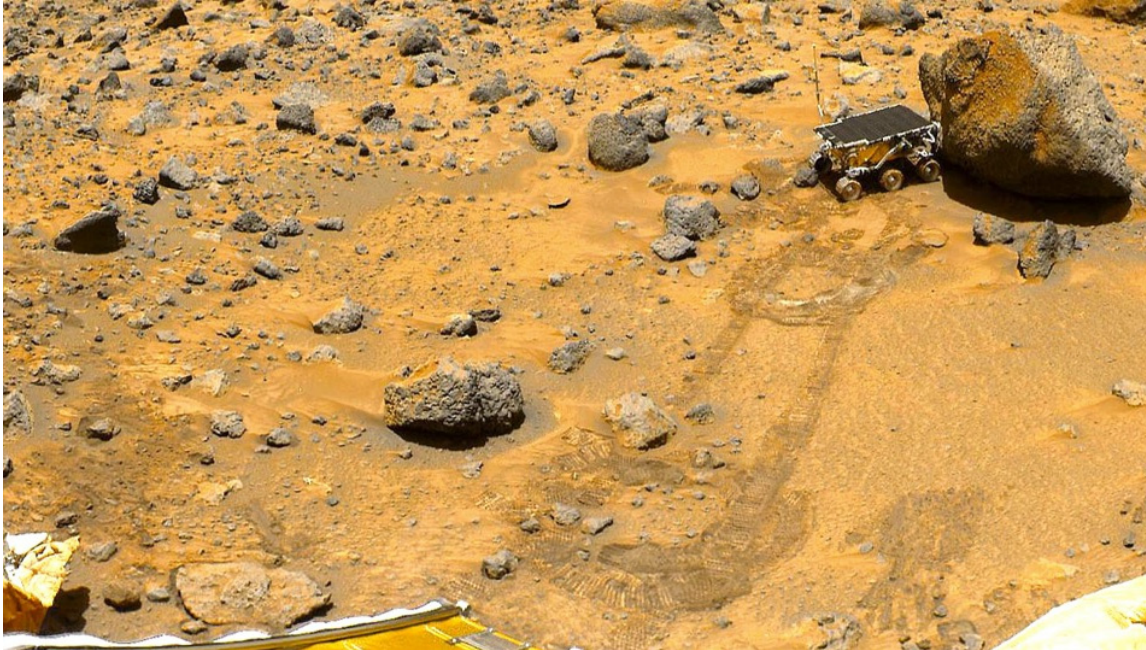
Figure 7. A view of Mars taken by the IMP camera showing the Sojourner Rover measuring the composition of Yogi rock. The deployed ramp that allowed access to the surface is shown in the lower left.
