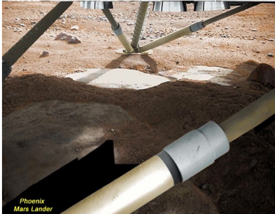
Figure 8. The robotic arm camera peered underneath the Phoenix lander to find that the thrusters (shown at the top of the image) had cleared away the overlying soil during final descent. From the curvature of the strut shadow the depth to ice can be estimated as 5 cm.
