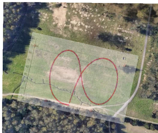
Figure 3. The perpendicular projection of trajectory I onto the XY plane against the background of the MUT training area
