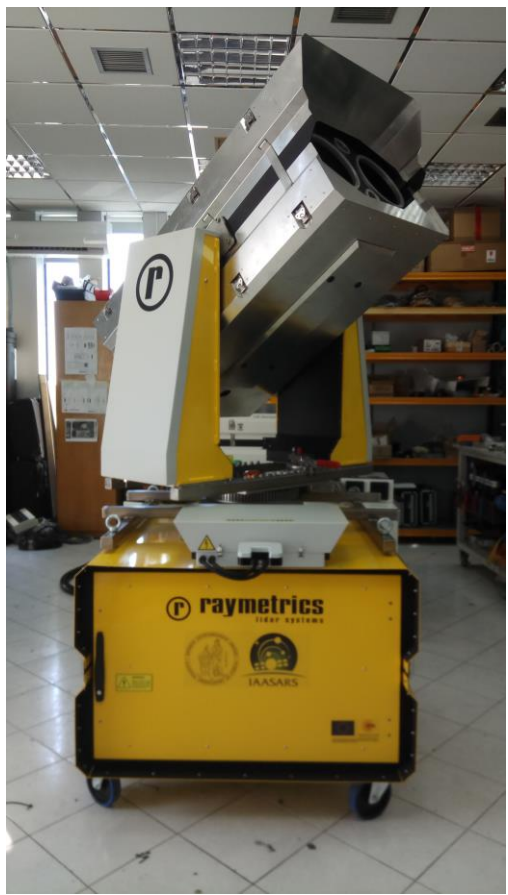
Figure 7. The WALL-E polarization lidar system for the detection of preferential particle orientation.
