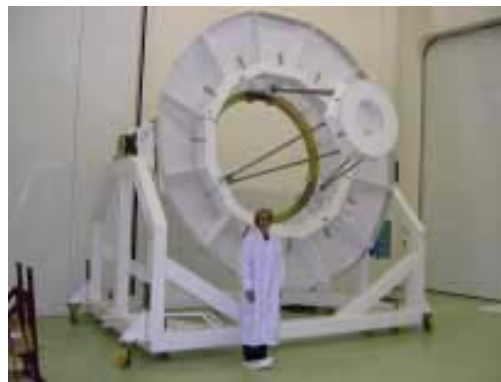
Figure 5-2: full-scale mock-up for handling and transportation rehearsal
