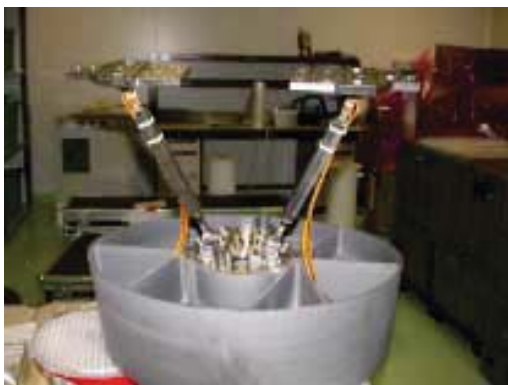
Figure 5-1: bipods connection mock-up
