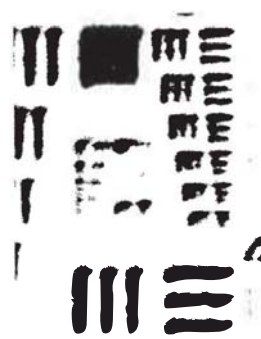
Figure 19. 1951 AFTP imaged with a 6µm pore Philips 33mm MCP in an image intensifier.
