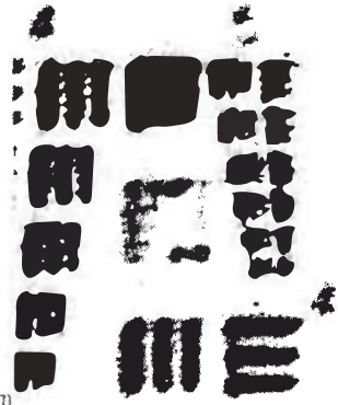
Figure 18. 1951 AFTP imaged with a 10µm pore Philips 33mm MCP in an image intensifier
