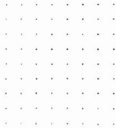
Figure 11. Image section of a 2 x 2mm, 10µm pinhole mask imaged on a 27mm² XDL detector.
