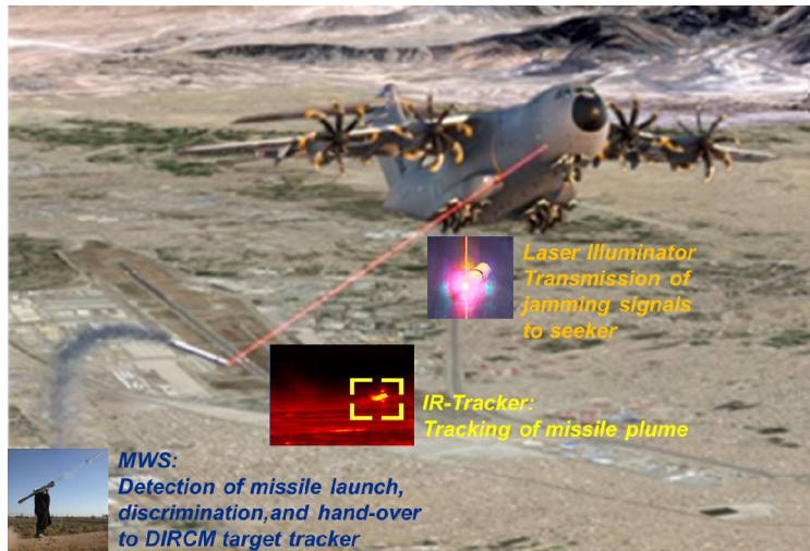
Figure 2 Basic operating principles of a DIRCM system (source: Diehl Defence)
