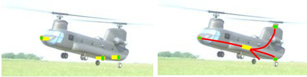
Figure 7 The distributed DIRCM concept; left: before implementation; right: after implementation; yellow boxes: lasers; green circles: frequency conversion sources; red lines: fibre delivery system (source: Ref. 61)
