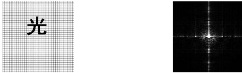
a. A image (Chinese character “光” + mesh) b. The frequency spectral distribution of the image
