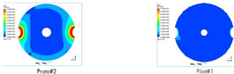
Fig.15 Simulation of thin deposition rate on the corrector mirror
