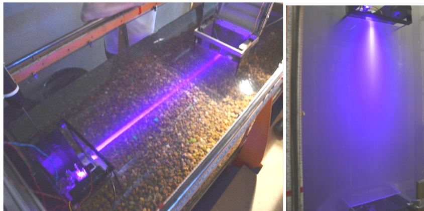
Figure 8: Full setup showing laser firing underwater and hitting detector 1m away with no Maalox added (left) and the scattering caused by adding 4 litres of Maalox (right).
