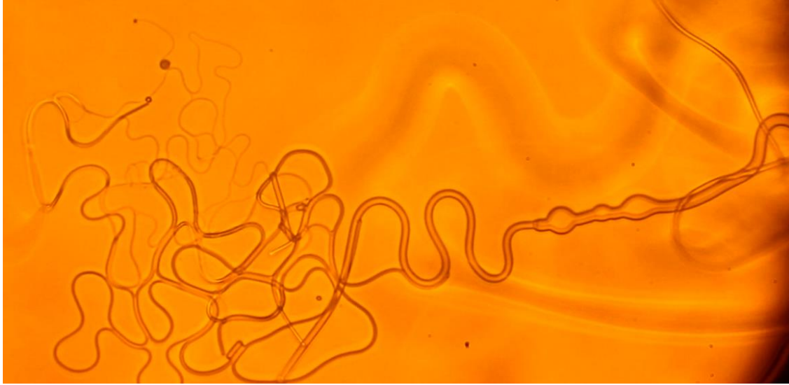
Figure 5. Snapshot from a video-movie, demonstrating the instability of the smectic-A fiber, caused by illumination with a pulsed doubled Nd:YAG laser. After having been exposed to the illumination, the fiber started to form wider areas (on the right) and a thinner fiber started to emerge from the fiber's end, moving towards the left side. The primary fiber shortened on this account, whereas the overall structure became longer and thinner. We can also see that thinnest fibers adhere to each other and form Y-junctions (left).
