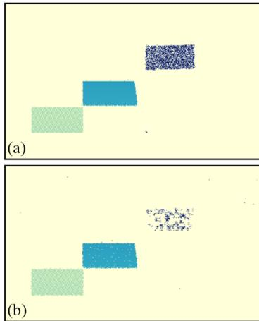
**Fig. 10** Range images with modified FOM measure and  $Q_{\max} = 3$ . (a) 0-dB transmitted power, detection threshold 1, and FOM threshold 9. This can be compared to Figs. 4(a) and 4(b). (b) -3 dB transmitted power, detection threshold 0.7, and manually tuned FOM threshold 42. The result can be compared to Fig. 7(b).
