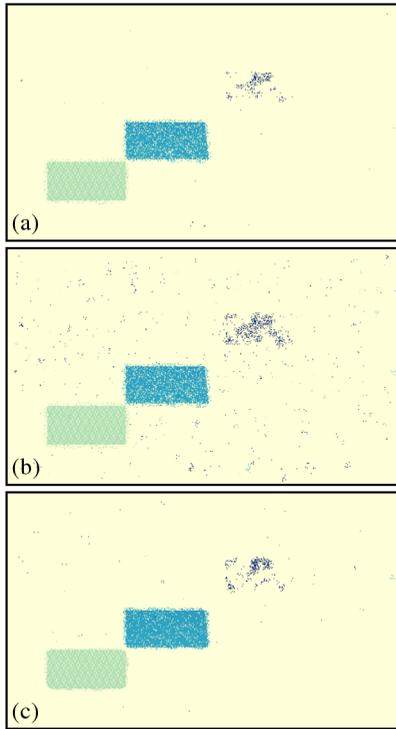
**Fig. 8** Range images with  $-4.8$ -dB transmitted peak power and  $3$ -mrad angular neighborhood size. (a) Detection threshold  $0.8$  and FOM threshold  $50$  (automatic). (b) As above, but FOM threshold  $44$ . (c) Detection threshold  $0.7$  and FOM threshold  $93$  (automatic).
