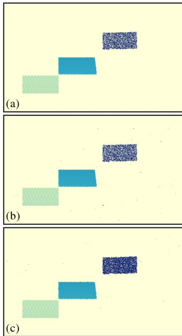
**Fig. 4** Range images with 0-dB transmitted peak power and 1.5-mrad angular bin size. The color-scale and the field of view are the same as in Fig. 3(a). (a) Detection threshold 1 (3.5 times the RMS noise) and FOM threshold 8 (automatic). (b) FOM threshold 6. (c) Detection threshold reduced 0.8 and FOM threshold 20 (automatic).
