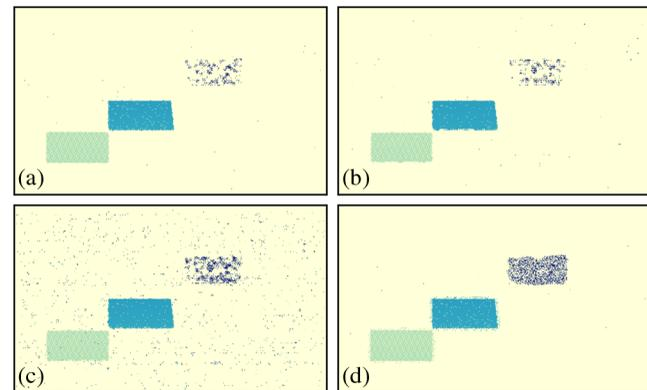
**Fig. 7** Range image with  $-3$ -dB transmitted peak power. (a) Detection threshold 0.8, 1.5 mrad angular neighborhood size and FOM threshold 20 (automatic). (b) Detection threshold 0.7 and FOM threshold 34 (automatic). (c) As (b), but with FOM threshold 30. (d) Detection threshold 0.8, 3 mrad angular neighborhood size and FOM threshold 50 (automatic).
