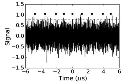
**Fig. 6** Typical return signal from the far object in the case with  $-3$  dB transmitted peak power. The dots above the graph mark the positions of expected return pulses, and the dashed line shows the detection threshold 0.8 used in Fig. 7(a).
