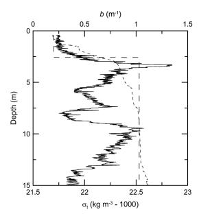
**Fig. 5** Profiles of density,  $\sigma_t$  (short-dashed line), a rough two-layer approximation to  $\sigma_t$  (long-dashed line), and optical scattering coefficient b (black line) at a wavelength of 532 nm. The measurement location was the northernmost of the two *in situ* measurements marked in Fig. 4. The total water depth at this location was 19.1 m.
