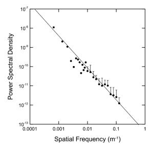
**Fig. 7** Example of measured power spectral density of lidar return along a layer as a function of spatial frequency. For clarity of presentation, spectral values have been averaged for wavelengths less than 100 m and the positive error bar represents one standard deviation of the initial values. The line is a -5/3 power law.
