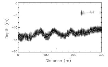
**Fig. 6** Example of the relative lidar return across an internal wave (white to black represents 0 to 1) as a function of distance along the flight track and depth. Each lidar profile has been normalized by its maximum value, and the depth of that maximum is plotted as a white line.
