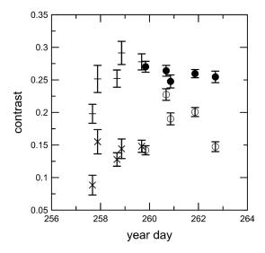
**Fig. 8** Optical contrast by flight as a function of year day, 2011. Symbols denote linear cross-polarized (+), linear co-polarized ( $\times$ ), circular cross-polarized ( $\bullet$ ) and circular co-polarized ( $\bigcirc$ ) values. Error bars denote  $\pm$  one standard deviation of the values measured during each flight.
