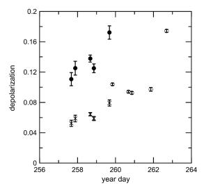
**Fig. 9** Layer depolarization by flight as a function of year day, 2011. (x) is linear depolarization, ( $\bigcirc$ ) is circular depolarization, and ( $\bullet$ ) is circular depolarization predicted from the measured linear depolarization. Error bars denote  $\pm$  one standard deviation of the average of each flight.
