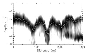
**Fig. 3** Example of the relative lidar return across an internal wave (white to black represents 0 to 1) as a function of distance along the flight track and depth. Each lidar profile has been normalized by its maximum value, and the depth of that maximum is plotted as a white line.
