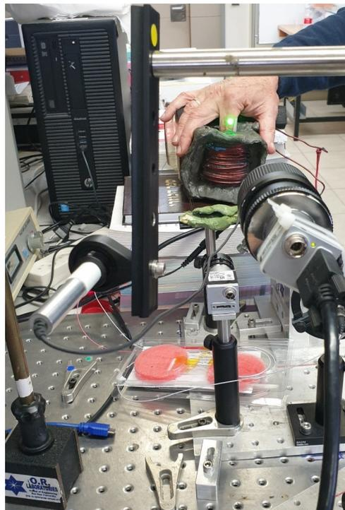
**Fig. 3** Experimental setup for blood glucose sensing.
