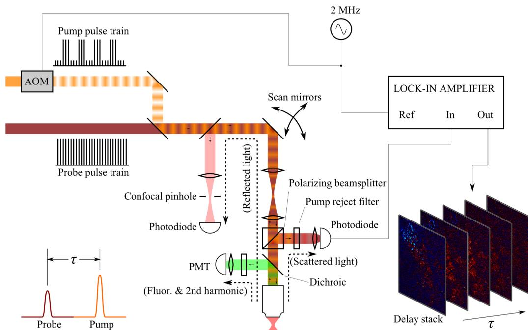
**Fig. 1** *In vivo* pump-probe microscope combining the following modalities: confocal reflectance; multiphoton autofluorescence and second-harmonic generation (SHG); and pump-probe microscopy.
