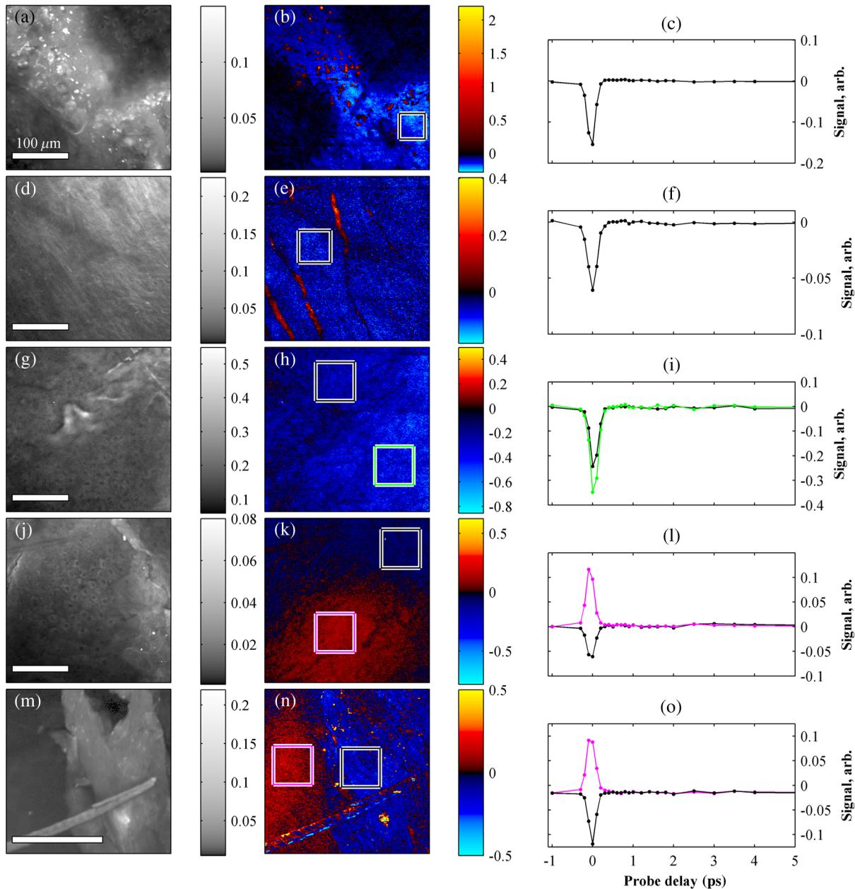
**Fig. 7** Examples of instantaneous “background” signal in pump-probe images. Left column: multiphoton fluorescence/SHG. Middle column: pump-probe image at time-overlap. Right column: pump-probe signal for highlighted regions of interest. Scale bars 100  $\mu\text{m}$ . Acquisition times: (a–l) 3 min /  $256 \times 256 \times 26$  delay stack; (m–o) 6 min for a  $256 \times 256 \times 26$  delay stack.
