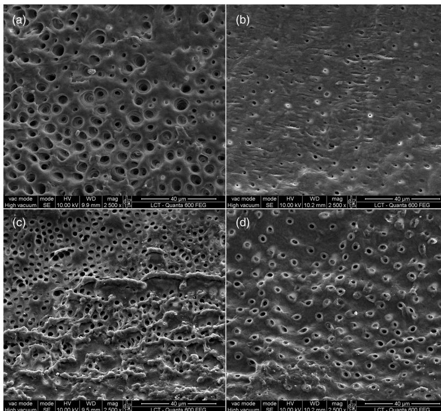
**Fig. 1** Composite scanning electron microscope (SEM) images of dentin. Control group with no surface changes (a); neodymium group (Nd:YAG laser) showing melting and resolidification of dentin surface (b); diode group (diode laser) also showing melting and resolidification but in a different pattern (c); erbium group (Er:YAG) showing ablation of the dentin surface (d).
