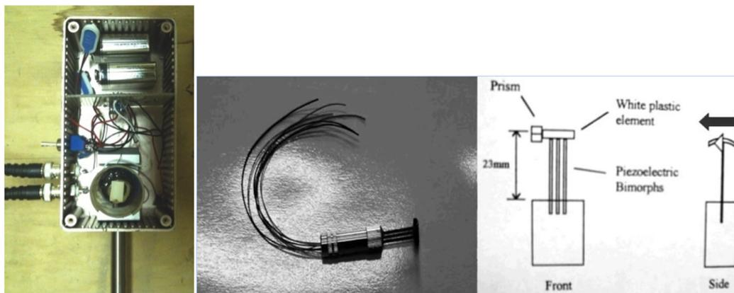
Fig. 4 OMT simulator. The small prism attached to the plastic disc is used during calibration of the simulator.
