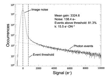
**Fig. 2** A measured PHD from a CCD201 with 604 multiplication elements operating at a gain of  $3300\times$ . The histogram shows the distribution of values measured in the image, and it can be seen that since most pixels have no signal that the gaussian read noise dominates at low signal levels. The plot includes a fit to the read noise and the extrapolated distribution of amplified events. The vertical dashed line shows the  $5\sigma$  threshold above which events are unambiguously detected.
