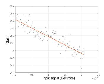
**Fig. 14** Measured electron multiplying gain as a function of signal input to the gain register at a gain of 25×.
