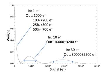
Fig. 1 Three theoretical PHDs for an EMCCD with 604 multiplication elements operating at a gain of  $1000 \times$  with 1, 3, and 10 electron input. The simulation does not include shot noise in the input signal.
