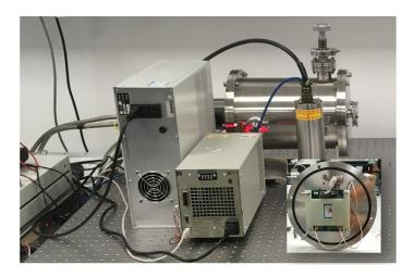
**Fig. 8** The CEI test camera utilizes a 1 MHz XCam XCU-A programmable controller coupled to a custom vacuum cryostat. The headboard and CCD, cooled by a Polycold Cryotiger to –105°C, is shown in the inset. An x-ray source is incorporated inside the vacuum for use in charge transfer calibration.
