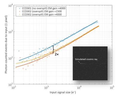
**Fig. 13** A comparison of the CCD301 and CCD302 register response to a single bright input pixel in photon counting mode. The figure shows the number of pixels after the bright pulse that would be counted as photons above the counting threshold. The inset shows an example "simulated cosmic ray," which is the result of a single bright pixel pulse to the gain register operating at high gain. Trailing pixels result from trapped charge at the register surface oxide due to the amplified signal.
