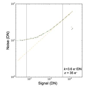
Fig. 11 A photon transfer curve for the CCD302 in the JPL 10 MHz camera.
