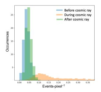
**Fig. 5** A comparison of noise in image row pixels with cosmic rays before the cosmic ray is detected (blue), underneath the tail (orange), and after the tail has faded (green). These reveal that the cosmic ray tails enhance the background significantly even in regions hundreds of pixels after the cosmic ray is detected.
