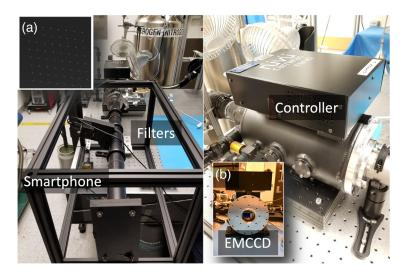
**Fig. 9** (a) A view of the smartphone projector system used for EMCCD characterization at JPL. Inset of panel A shows an example image from the projector. (b) The JPL test camera utilizes a 10-MHz NuVu CCCP programmable controller coupled to a custom vacuum dewar and is cooled by liquid nitrogen to  $-105^{\circ}$ C. Inset of panel B shows a test EMCCD in the commercial dewar.
