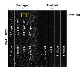
**Fig. 15** A 100-hr photon counted CCD301 image comprised of 100-s frames of data. A line image from the projector illuminates row 960 near the top of the array. The pixel designs are mirror-imaged on the left and right sides of the image with the shielded right hand side providing a control. The 95% dark level measured after irradiation is overlaid on each design on the left side of the figure. The yellow rectangle shows an example extraction area for the irradiated notch-design data.
