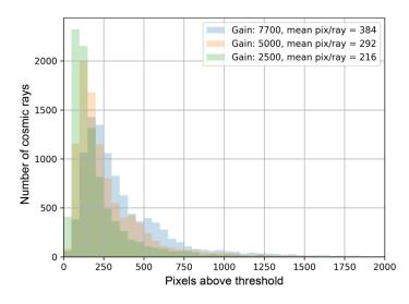
**Fig. 3** The distribution of cosmic ray tail contamination (number of pixels above the five sigma photon counting threshold) versus gain for the commercial CCD201.
