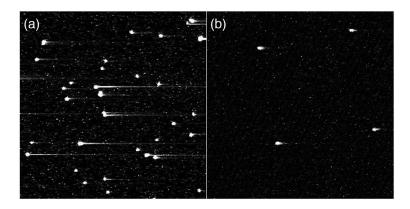
**Fig. 21** A comparison of cosmic ray tails observed in the lab with the camera operating at high gain (>1000×). (a) A 256 × 256 image section from the CCD201 and (b) the CCD311 under similar conditions. The operating temperature was  $-105^{\circ}$ C. The improvement is quite significant with tails in the commercial sensor example of over 100 pixels and only 40 pixels in the flight design as a result of the overspill.
