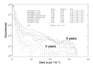
**Fig. 16** Dark current histograms extracted from the photon counted image shown in Fig. 15. Each histogram is extracted from a different design region as labeled. The shielded half of the array provides the "0 year" beginning of life data while the irradiated half represents the 5-year lifetime goal at L2.
