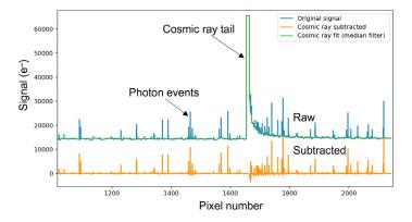
**Fig. 4** The blue traces show a row of raw photon data with a representative cosmic ray tail. The green trace shows a fit to the tail generated by a median filter. The orange trace shows the fit-subtracted data, revealing an excess of events in the underlying pixels.
