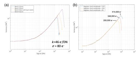
Fig. 10 (a) Photon transfer curves from CEI in the 1 MHz camera for each of the four image pixel designs contained in the CCD301 test sensor. (b) Photon transfer curves for the CCD301 register, which is common to all of the image pixel designs, at three clock voltages.
