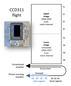
**Fig. 20** The flight CCD311 EMCCD incorporates the image pixel notch feature from the CCD301 and the gain register overspill from the CCD302. It utilizes a commercial aluminum nitride carrier bonded into a nickel-plated invar package. The CCD311 is pin compatible with the commercial CCD201.
