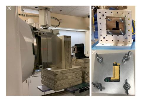
**Fig. 7** (a) The proton irradiation test configuration at Loma Linda Medical Center. (b) A close-up of the EMCCD and test shield. (c) A test package behind the shield (without silicon) revealing the unshielded half of the package.
