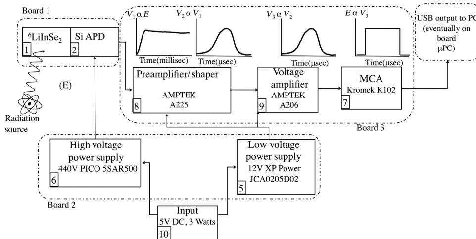
**Fig. 3** Block diagram of the detection system including (1)  $\text{LiInSe}_2$  crystal, (2) Si-APD, (7, 8, 9) associated electronics for signal processing, and (5 and 6) power supplies. The main information extracted from each signal is the height of the pulse, which is linearly proportional to the energy of the ionizing particle detected. Labeling of components is the same used in previous figures.
