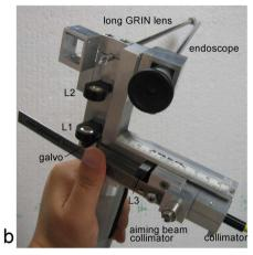
**Fig. 2** (a) Schematic diagram of a GRIN lens rod–based dynamic focusing swept-source OCT system. (b) Design of the probe. DM—dichroic mirror; Ls are lenses.
