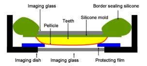
**Fig. 3** Imaging dish specifically designed for salivary pellicle imaging. To protect against dehydration and mechanical irritation of the developing salivary pellicle, the imaging dish border was sealed using silicone (top), and the window border was protected by  $100-\mu$ m-thick plastic film. The gap between the imaging glass and the salivary pellicle assures an intact and unchanged salivary pellicle throughout imaging.
