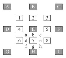
Fig. 1 Fractional pixel search positions.
