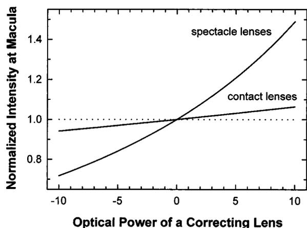
**Fig. 12** Relative variation in the laser light intensity at the retina with the optical power of correcting spectacles or contact lenses. These curves should be used on a regular basis for adequate correction of MP Raman data when the subject has used his or her lenses during MP measurements.
