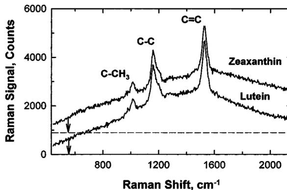
**Fig. 3** Resonant Raman spectrum of methanol solution of zeaxanthin and lutein measured under excitation with a 488-nm argon laser line. The horizontal dashed line indicates zero for the Raman spectrum of zeaxanthin, which was shifted by 900 counts for the sake of clarity.
