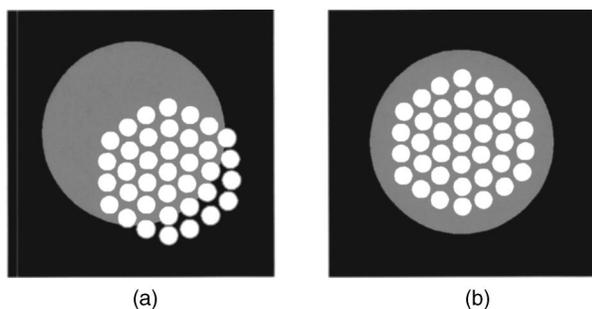
**Fig. 6** Procedure for alignment of the Raman instrument with the optical axis of the subject's eye. The subject sees two colored light patterns when looking into the instrument: a weak blue circular disk from the argon laser fiber (shown in gray) and a weak red polka-dot pattern originating from an LED-illuminated light-collection fiber bundle. Alignment is achieved when the subject moves his or her head so that both patterns overlap. (a) Misaligned; (b) aligned.
