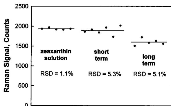
**Fig. 11** Repeatability of Raman measurements. The left part represents data for zeaxanthin solution in a model eye. The central and right data represent the short-term and long-term repeatability of macular pigment measurements for two different subjects. The Raman intensities for the long-term dataset were measured over a 2-week period in five sessions.
