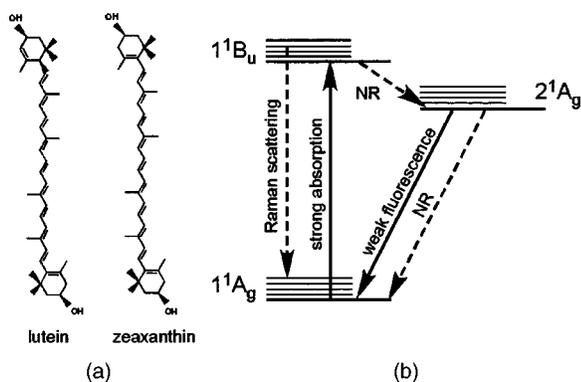
**Fig. 1** (a) Chemical structure of lutein and zeaxanthin molecules. They differ in the location of the additional C=C bond in one ionone ring. (b) Energy-level diagram of long-chain carotenoid molecules with optical and nonradiative transitions.
