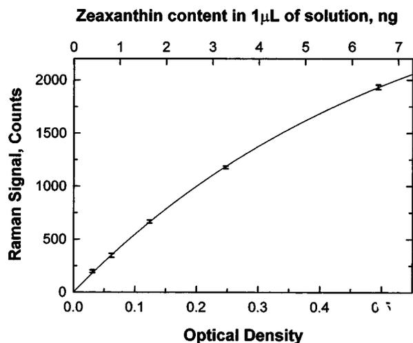
**Fig. 10** Calibration curve of the MP Raman detector linking the instrument reading with the carotenoid content in a human macula. The curve was obtained using a model eye discussed in the text containing zeaxanthin dissolved in methanol. The sampling volume, 1  $\mu\text{l}$ , corresponds to a 1-mm-diameter spot at a macula and contains carotenoid typical for a human macula.
