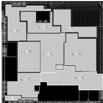
Figure 4: Hierarchical approach allows IP blocks already analyzed by design teams to be skipped at SoC level using a “NO LPC” marker
