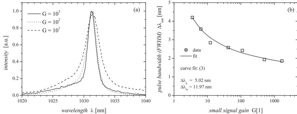
Figure 5. Influence of gain narrowing in Yb:YAG; (a) output pulse spectra at a small signal gain of 10,  $10^2$ , and  $10^3$ , (b) output bandwidth (FWHM) vs. small signal gain of the Yb:YAG multi-pass amplifier.
