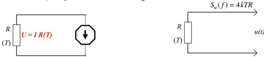
Figure 1. Left: Resistor thermometer; the  $R(T)$  function must be known and a biasing DC current, which is heating the thermometer and causes error, and precise current and voltage measurements are needed. Right: The usual Johnson-noise thermometry; the  $R(T)$  function is not needed but the resistance value  $R$  must be known and precise current and voltage measurements are needed.
