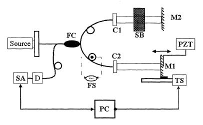
Figure 2: Experimental setup for ballistic waves attenuation through a scattering background. FC fiber coupler; C1, C2 collimaters; SB scattering background; M1, M2 mirrors; PZT piezolectric transducer; TS translation stage; FS fiber stretcher; D detector; SA spectrum analyzer; PC personal computer.
