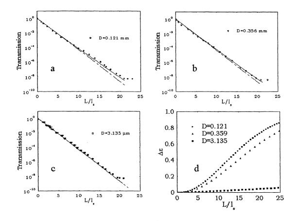
Figure 3: Experimental results for ballistic attenuation through media of different particle sizes, as indicated. In a, b, c, the dashed lines reprezent exponential decays; the continuous lines are given by Eq. 2. In d,  $\Delta \varepsilon$  is the relative difference between the Lambert-Beer law and Eq. 2.
