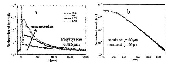
Figure 5: OPS experimental results for media of different concentrations (a) and an example of data fitted with Eq. 4 (b).
