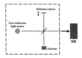
Figure 4: Backscattering configuration for optical pathlength spectroscopy.
