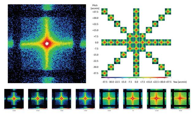
Figure 3 Measurements of the MXT-MOP-FM at Al-K (1.5 keV): (top left) a grid of  $3 \times 3$  TRoPIC images combined to study the cross arms of the PSF in detail, (top right) a so-called focal plane map obtained to study variation of the PSF and efficiency of the optic on-axis as well as for a grid of off-axis angles. (bottom) the PSF as a function of energy is shown from left to right C-K, O-K, Cu-L, Al-K, Ag-L, Ti-K, Fe-K, Cu-K.
