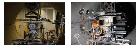
Figure 7 The PANTER thermal shroud and its MLI covering are visible above the MXT-FM. The MXT-FM model in the chamber, (left) with the MOP cover removed, prior to closing the chamber door and pumping down. Photo is taken looking from the direction of the X-ray source. (right) The detector end of the MXT inside the chamber, shortly before closing the chamber and pumping down. The PANTER thermal shroud and its MLI covering are visible above the MXT-FM. Photo is taken facing the X-ray source.
