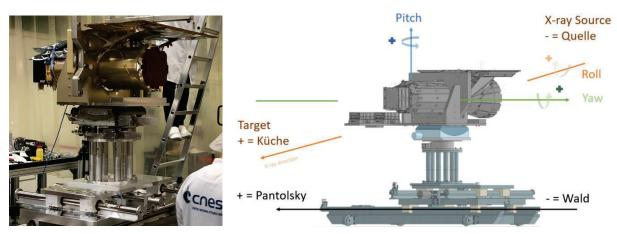
Figure 5 (left) Photograph showing the SVOM-MXT-PM model telescope being mounted onto the PANTER manipulators in the grey area. (right) shows the coordinate system used during the telescope tests.
