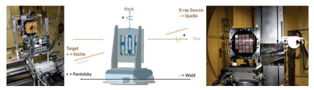
Figure 1 SVOM-MXT-MOP optics in the PANTER vacuum chamber, view from the source toward the detector: (left) the Bread-Board (BB) and (right) the Qualification Model (QM) models are shown. (center) shows the coordinate system used in PANTER during the optics measurement campaigns. During the BB measurements, the Position Sensitive Proportional Counter (PSPC), a ROSAT flight spare, was also used for measurements together with the TROPIC pnCCD camera.
