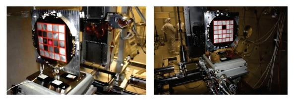
Figure 2 SVOM-MXT-MOP optics in the PANTER vacuum chamber, view from the source toward the detector: (left) the Flight Model (FM), and (right) the Flight Spare (FS) models are shown.
