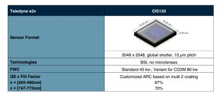
Figure 9. Main characteristics of the CIS-120 silicon CMOS detector from Teledyne-e2v.
