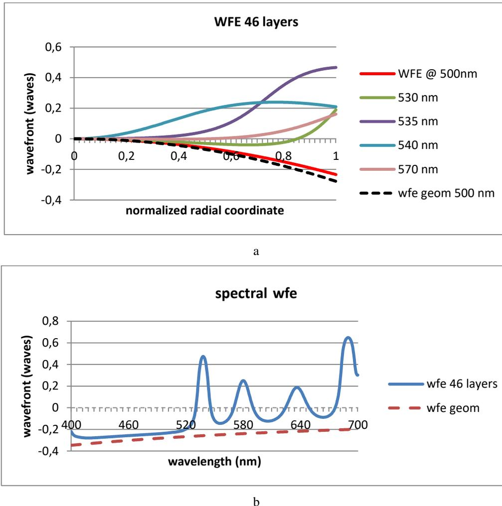
Figure 5. Variation of the actual wavefront with wavelength, compared to the geometrical wavefront (dashed line): a) radial profile at some wavelengths, assuming 2% thickness decrease along the radius, b) spectral profile in which the correspondence with the upper graph at the maximum radial coordinate can be verified.
