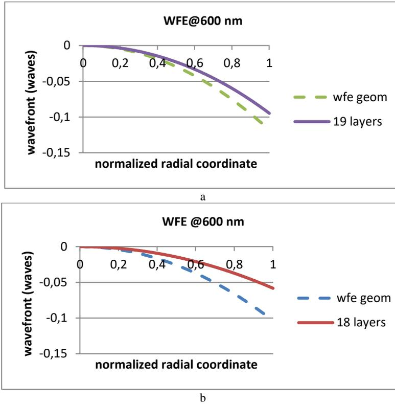
Figure 2. Wavefront of a) 19-layer and b) 18-layer high reflectance coating, compared to the geometrical wavefront (the radial coordinate equal to 1 corresponds to the minimum thickness reduced of 2%).
