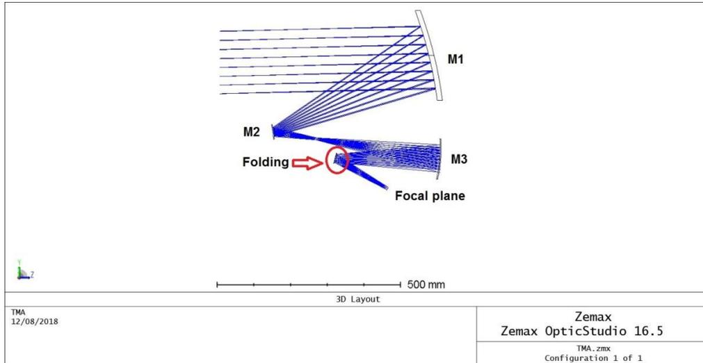
Figure 8. Layout of the TMA telescope
