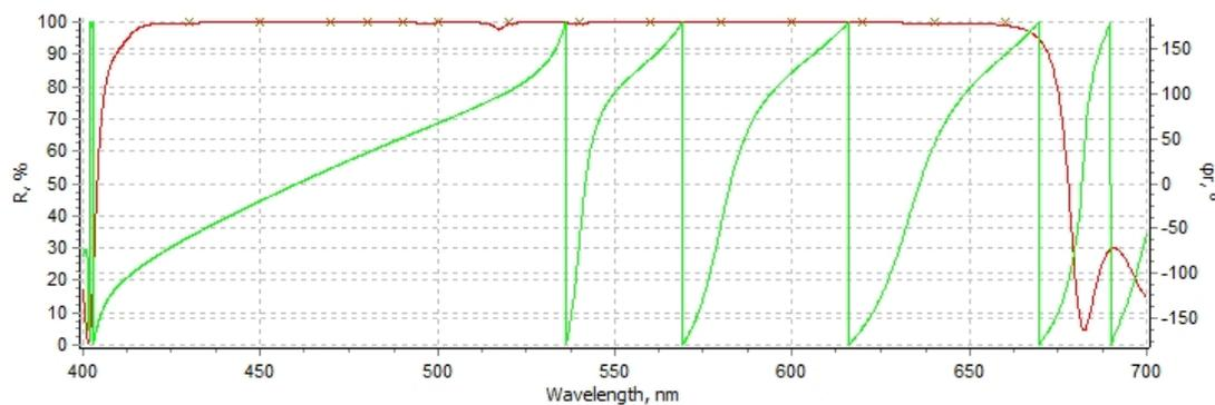
Figure 4. Reflected intensity (red) and phase (green) of a broadband mirror for the visible range, made of 46 layers of SiO<sub>2</sub> and Ta<sub>2</sub>O<sub>5</sub> obtained combining two q.w. stacks, with a total thickness of 3.47 μm.
