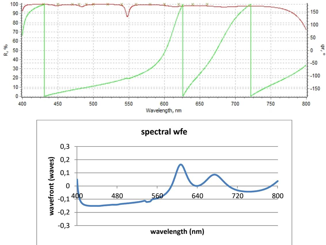
Figure 6. Spectral reflectance (red), phase (green) and wavefront of a 23-layer coating.
