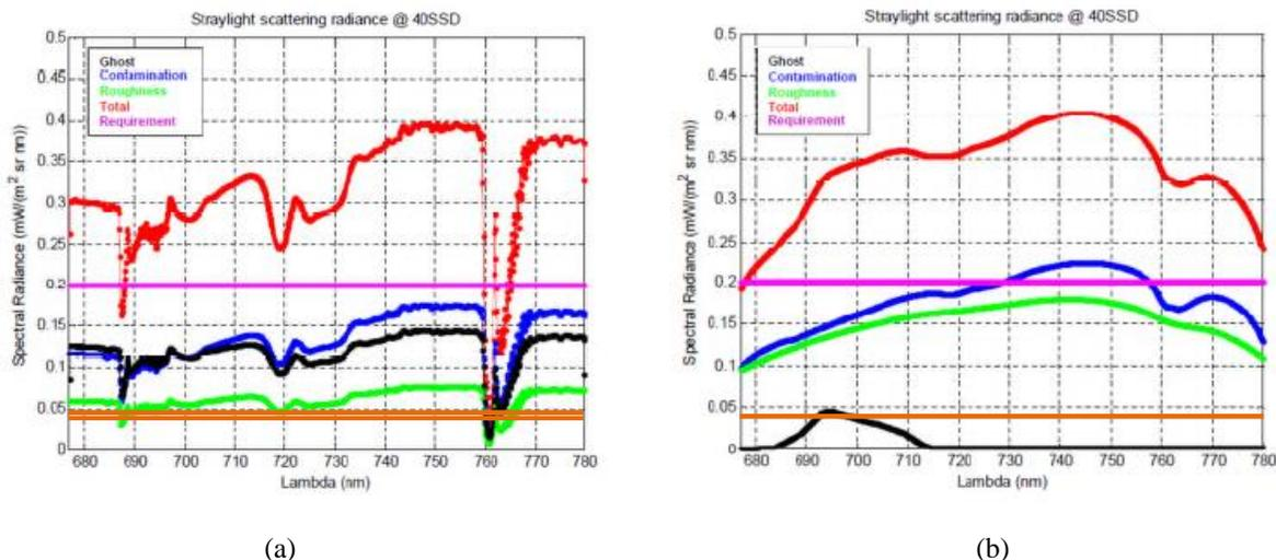
Figure 4: Computed straylight performance (a) telescope (b) HR spectrometer
