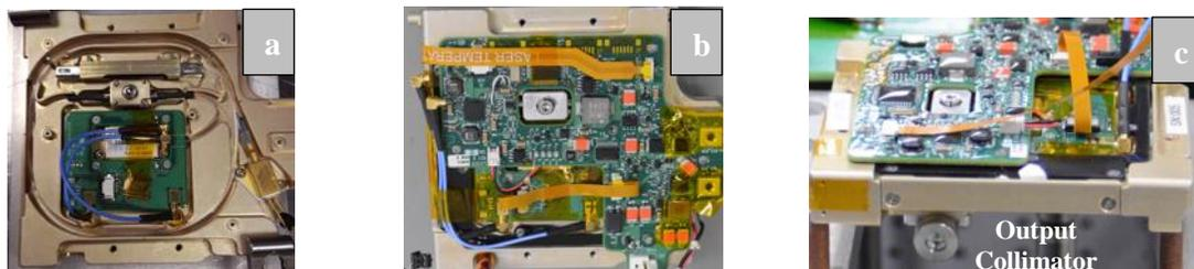
Fig. 6: Photos of the laser transmitter slice during build: (a) initial layout of components, (b) integration of laser control electronics and (c) output lens visible on underside, which also holds the fiber amplifier.
