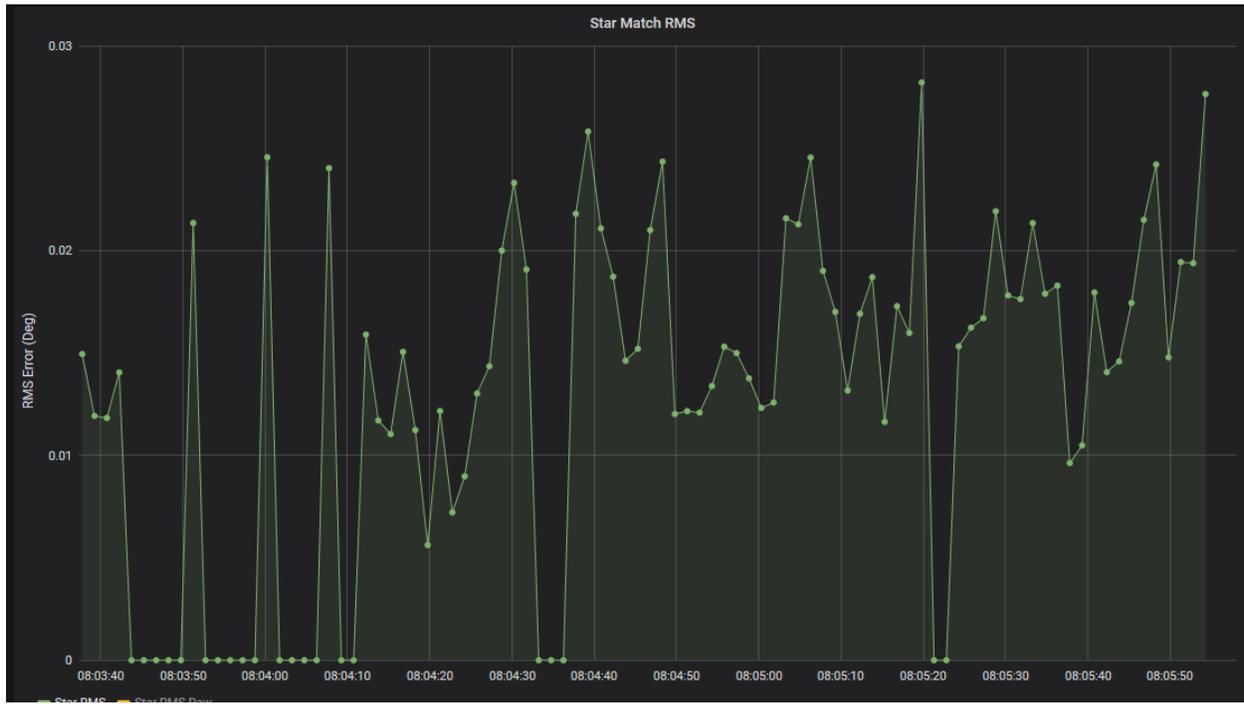
Fig. 3: Root Mean Square (RMS) errors of Star locations w.r.t. catalog geometry for four to eight matched stars. Note time intervals with fewer than four stars matched are mapped to zero RMS error on this plot.
