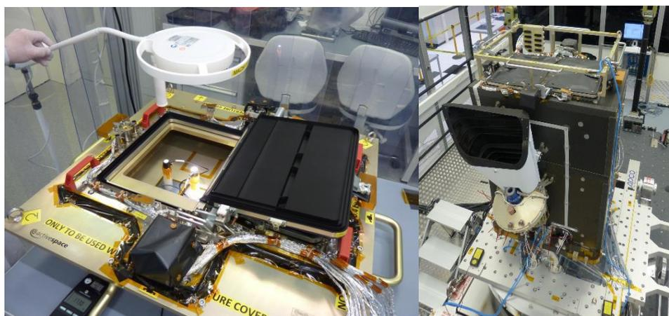
**Fig.7b:** Left: Aperture Cover Qualification Models Right: Calibration assembly and ACV QM assembled on the Instrument EM
