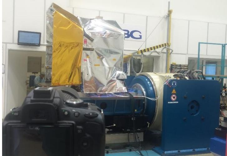
**Fig. 12:** OIM structure STM mounted on the vibration bench at IABG
